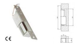
The R2 Electric Strike RIGHT is designed for remote opening of right and double-wing doors and gates, in co-operation with the door lock striker. It is made of aluminium alloys and powder-painted. It is designed to be mounted within a doorframe, in which it is possible to make a 28x31x119 mm mounting hole (draw on the right).
